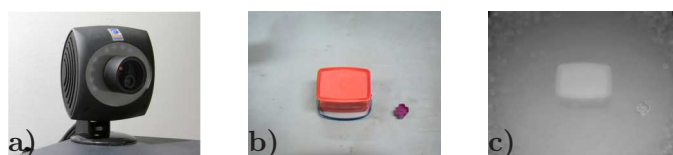
Figure 3.5 The robot's vision system: a) a closeup of the 3D camera; b) a color image of a red non-container captured by the camera when mounted on the robot; c) the depth image corresponding to b).
